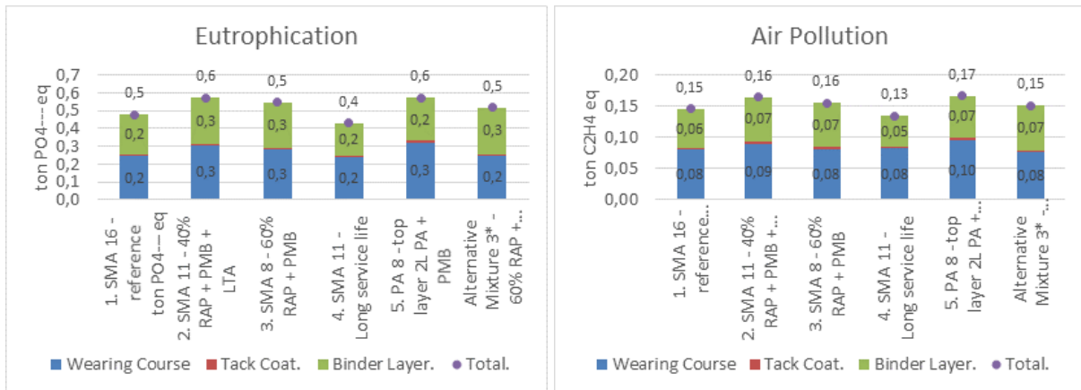
Figure 20: Results for the six scenarios, per layer. Top: results for Global Warming Potential; bottom left: results for Eutrophication; bottom right: the results for Air Pollution.
