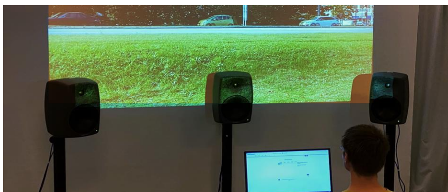
Figure 32: Listening room at FORCE Technology – sound is played from the stereo setup and the video is shown at the large screen. The assessors are answering questions on a PC.
