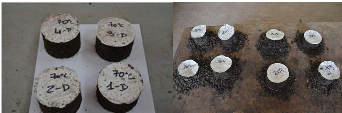
Figure 11: Marshall samples compacted at 70°C (left) and 20°C (right)
