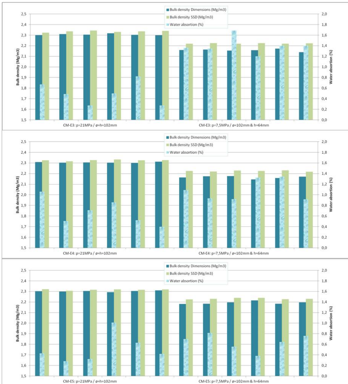
Figure 29 – Bulk density of cylindrical test specimens of bitumen emulsion stabilized materials
