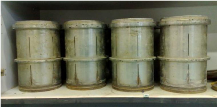
Figure 11 – 150 mm diameter slotted moulds
