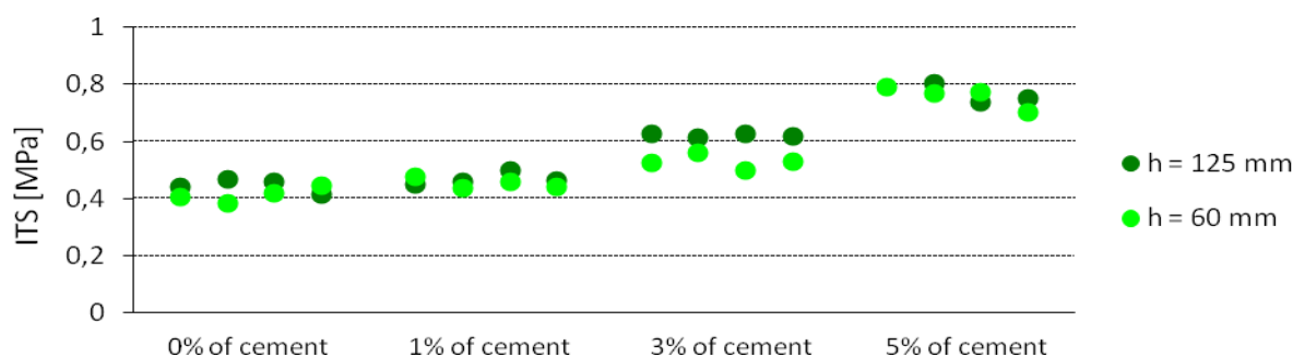
Figure 54: Comparison of indirect tensile strength and the height of test specimen for different mix designs
