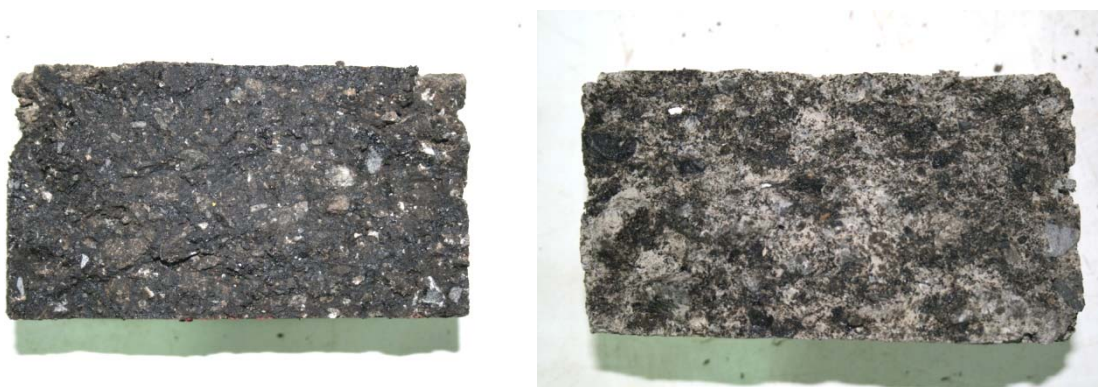
Figure 39. Specimens with bituminous emulsion (left) and foamed bitumen (right)
