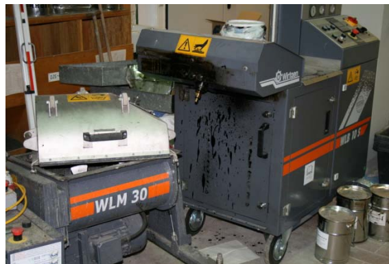
Figure 12. Wirtgen WLM30 pugmill mixer and WLB10S laboratory plant
