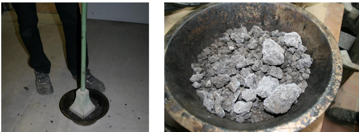
Figure 3: Breaking procedure for prepared specimens
