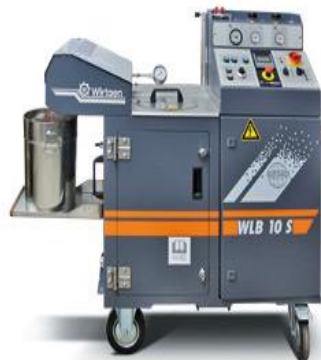
Figure 7: Laboratory device for production (generation) of foam bitumen
