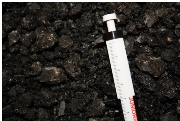
Figure 9: Multiple aged and crushed RAP
