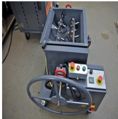
Figure 6: Detail of the two-shaft drum mixer WLM 30
