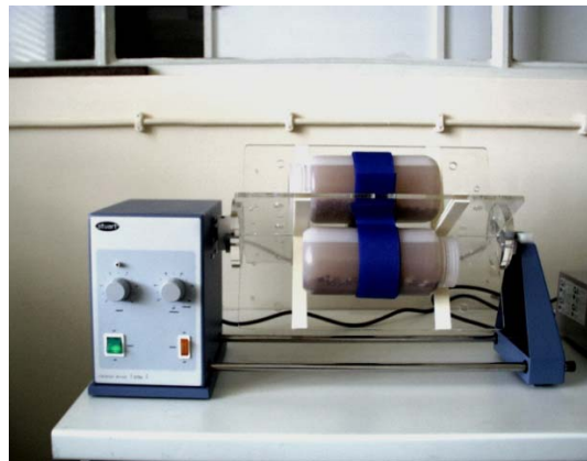
Figure 5: Batch leaching test (LNEC)
