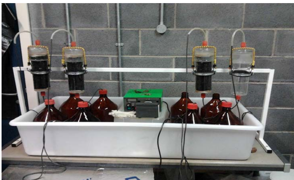
Figure 6: Percolation test set-up at UCD
