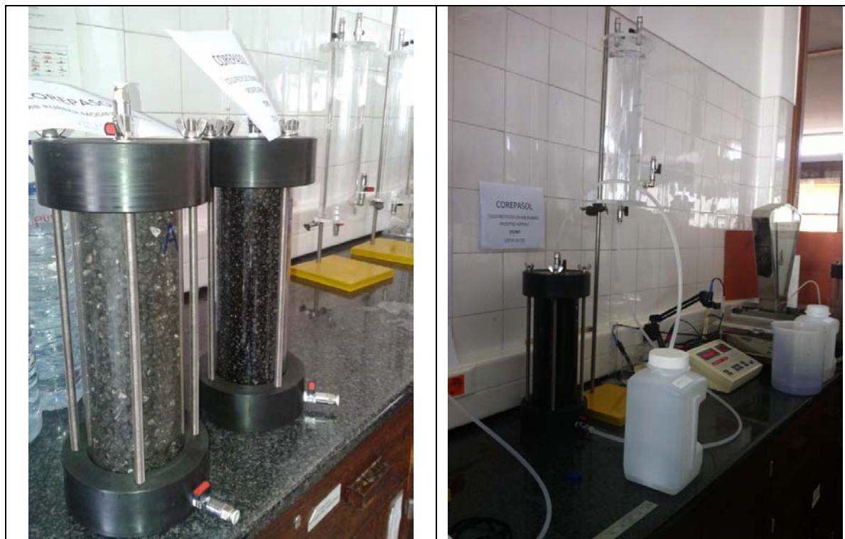
Figure 7: Percolation test set-up at LNEC: (a) Column with P2 (RAR) and column with P3 (RAR-BE); (b) Running percolation test on P3 (RAR-BE column)
