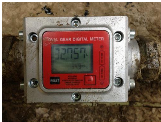
Figure 3-4: Gas oil consumption was measured at 30 s intervals throughout batching
